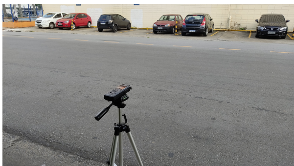
Figure 3: Setup for audio recording of traffic noise.
