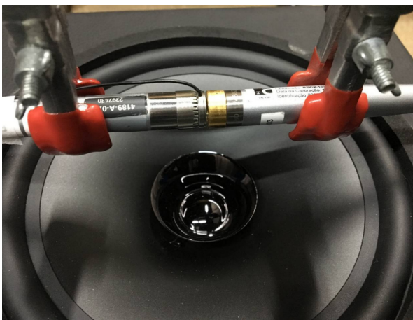
Image 3: Face-to-face microphone mounting, orthogonally to the sound wave direction, based on the configuration specified in IEC 61094-5.
