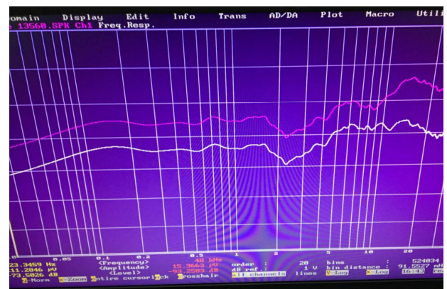
Image 4: Frequency response of reference and surface microphones in a face-to-face configuration, excited by a sine-sweep and processed by TST.
