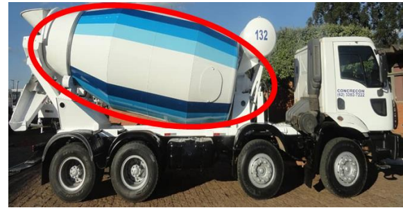
Figure 1 – Representation of the concrete truck's mixer.
