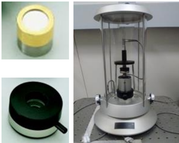
Figure 1: At left, above, a picture of a half-inch laboratory standard microphone; at left, below, a picture of a plane wave coupler for half-inch microphones; and at right, a picture of a pair of half-inch microphones connected by a coupler.
