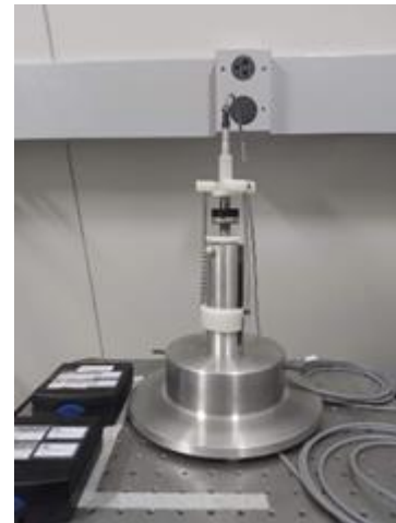
Figure 4: Picture of a half-inch microphone connected to a sound source (another microphone) by a coupler.
